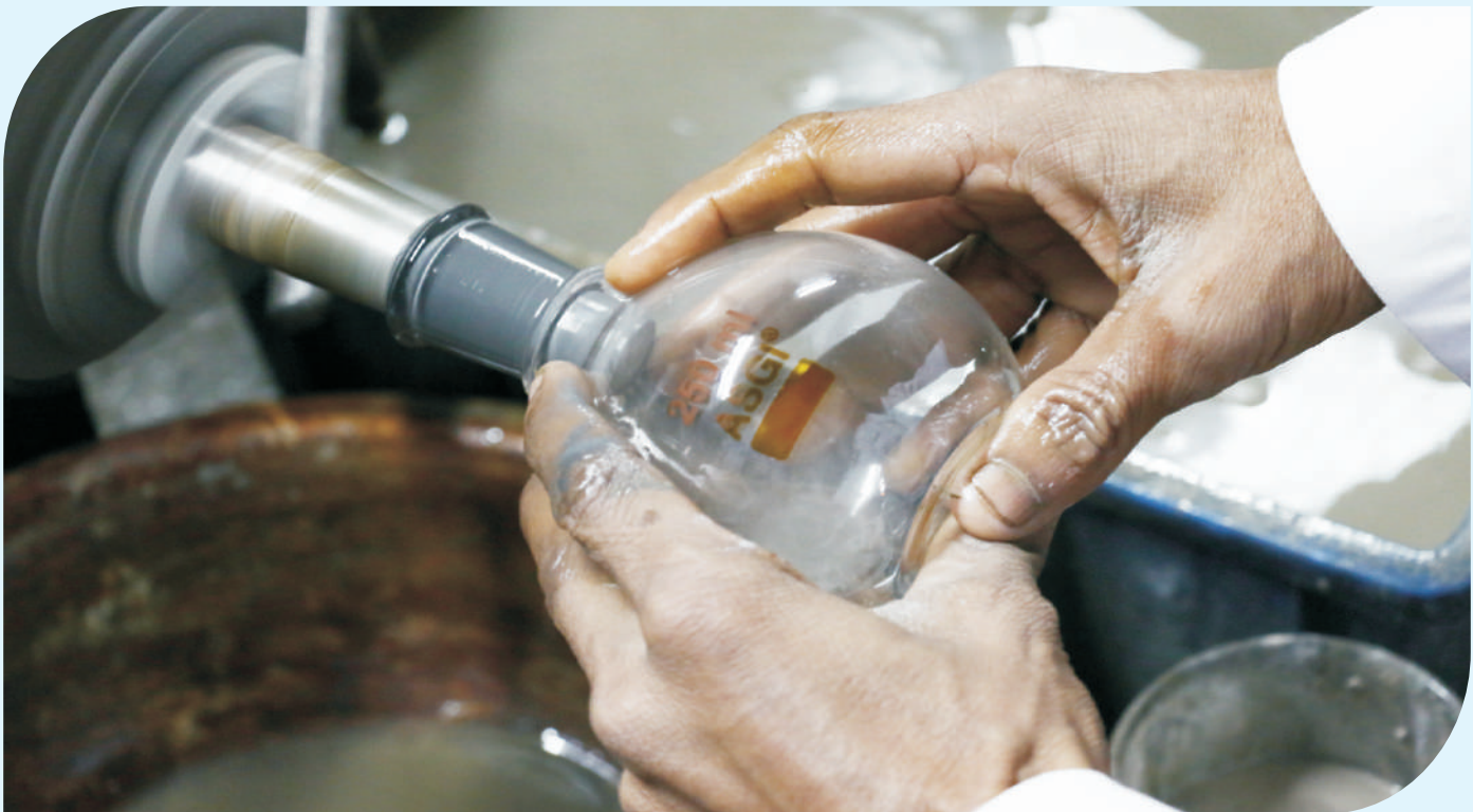
grinding & polishing of joints
